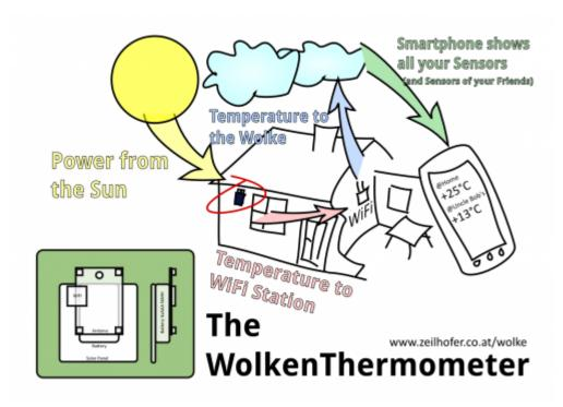
The aim is a compact sensor device with WiFi connection and a temperature sensor. Put it anywhere in the range of your WiFi at home, and read the measurement value on your smart phone from around the world. It runs on rechargable batteries in combination with a small solar panel and should work for many, many years.
