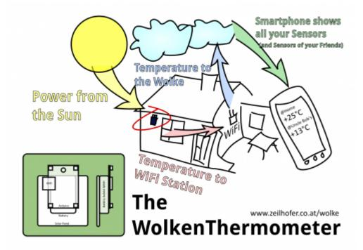
The aim is a compact sensor device with WiFi connection and a temperature sensor. Put it anywhere in the range of your WiFi at home, and read the measurement value on your smart phone from around the world. It runs on rechargable batteries in combination with a small solar panel and should work for many, many years.
