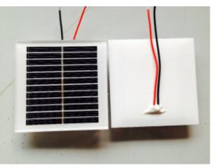
one transmit, including dailing into the WiFi needs about 10s, then we can send a packet every 240s = 4 minutes. In summer we get about 4 times the energy in a day than in a winter day. Which leads to a transmit period of 1 minute.
